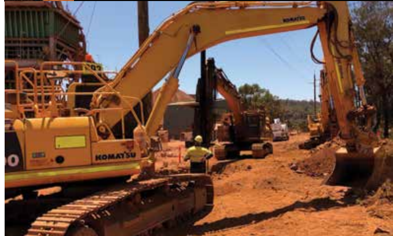
JSW Montabert Drill Rig drilling hard cap rock at South32 Worsley Alumina Boddington Bauxite Mine.
